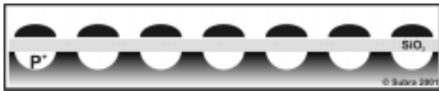
Fig. 5: Schematic diagram of CCD structure
